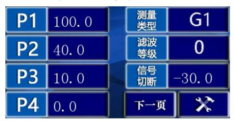
Note: The signal point setting value needs to meet the following requirements: P1>P2>P3>P4.
